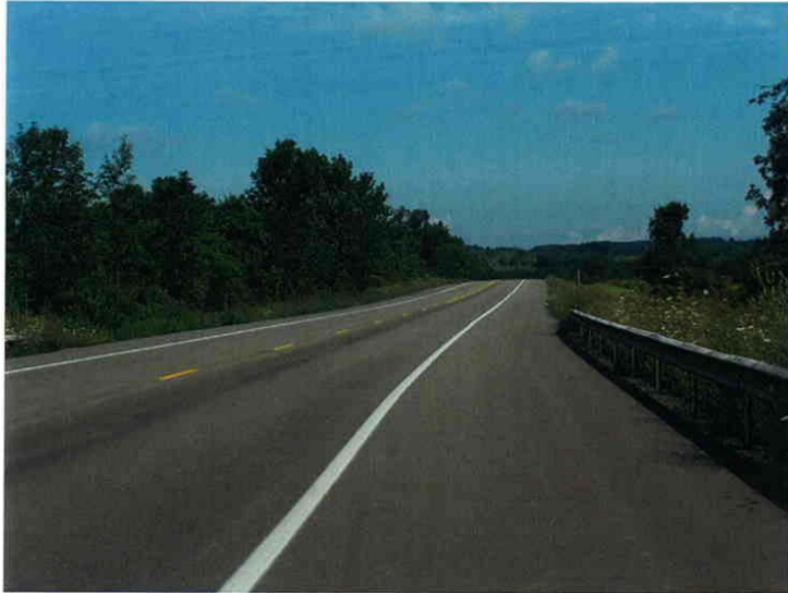
Photograph 11 Looking north on US Rt. 62, 3.5 miles north of the NY/PA boundary. There are two 11.5' wide lanes and 9' wide paved shoulders.
